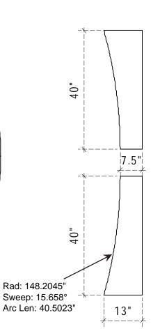
Concave Wing for P-Series 20' Unit includes (2) Bottom Panels and (2) Upper Panels
